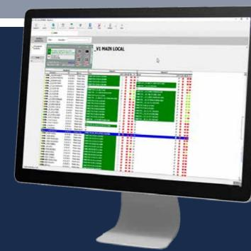
There are three versions: a free one in which two audiocodecs are shown per screen, another one in which all the codecs of a system or fleet are controlled from the same screen, and a third one in which, in a broadcasting network, the distribution of programs and contributions from affiliated stations, are managed, automatically or manually, with the support of an audio matrix.
